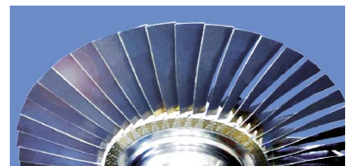
Gas Turbine Rotor
